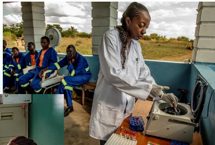
Centrifuge run on car battery
